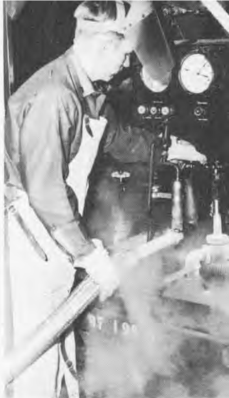
Personnel fill nitrogen cylinders, opposite and above. Below, 18-lb. oxygen converter produces same amount of breathable oxygen as two cylinders weighing 300 pounds.
