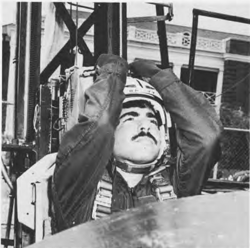
A future aircrewman prepares to pull the face curtain upon the command of "Fire," above. This action will explode a cartridge that will send him eight to twelve feet up the track.
