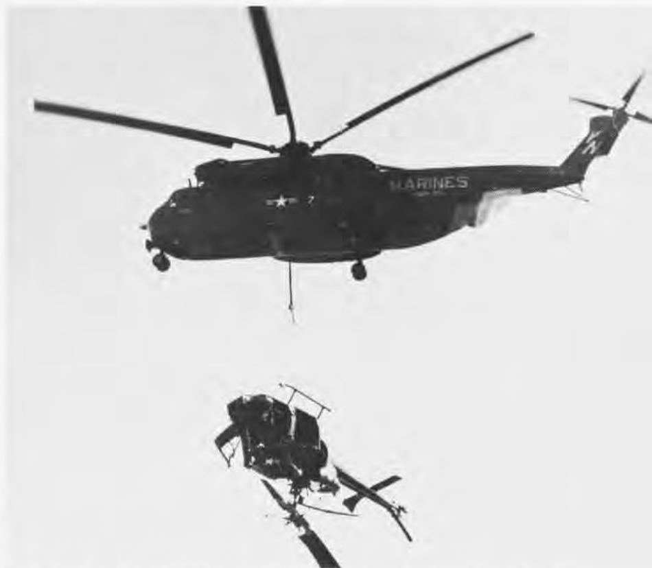
Not all aircraft come home right side up, as a wrecked H-1 is recovered by a Sea Stallion.
