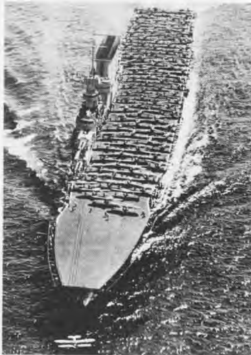
CV-3 launches its aircraft. Note short takeoff roll for forward aircraft. On the opposite page, Saratoga is tied up at NS Mayport.
