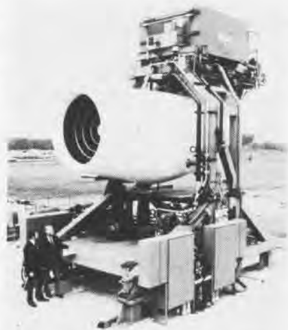
This 22,000-lb. thrust experimental quiet engine, developed by NASA's Lewis Research Center, Cleveland, is quieter than any engine in use on commercial jets. Test engine is housed in nacelle lined with special acoustic treatment to dampen sound, especially the higher frequencies which irritate people.
