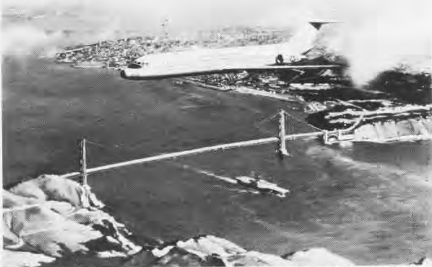
Navy has awarded McDonnell Douglas a contract for the purchase of five C-9B's plus spare part support. The new transport, depicted in this R. G. Smith painting, is a specially equipped, longer range version of the DC-9. The new version will be used for fleet logistic support.
