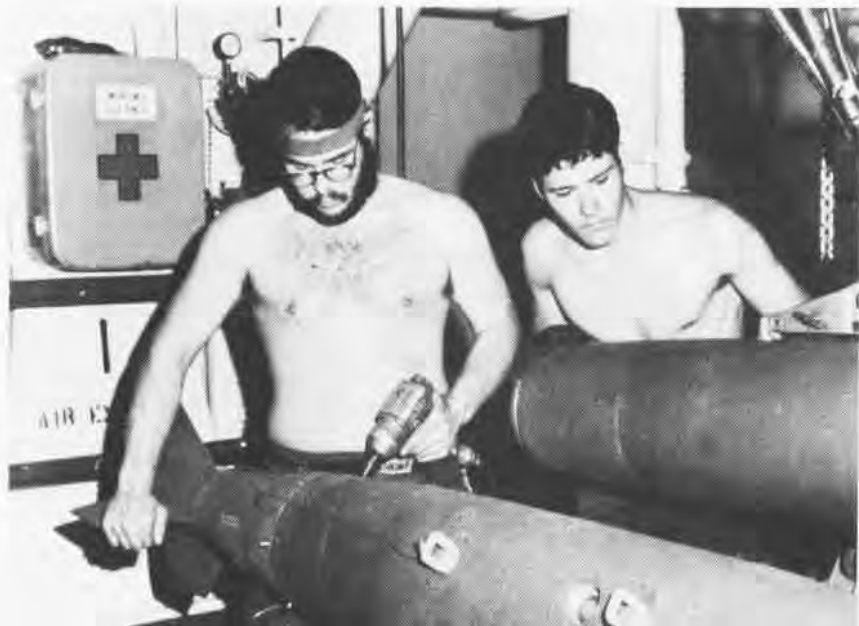
Prototype MER/TER tester is used during first fleet evaluation aboard Enterprise, above. Fins, electrical fusing, booster adapter and arming wires are installed during bomb assembly below decks, below. Enterprise AOs attach Mk 82 bombs to a MER, opposite top, and a flight deck bomb loader with his HLU-196 awaits delivery of a preconfigured load, right.
