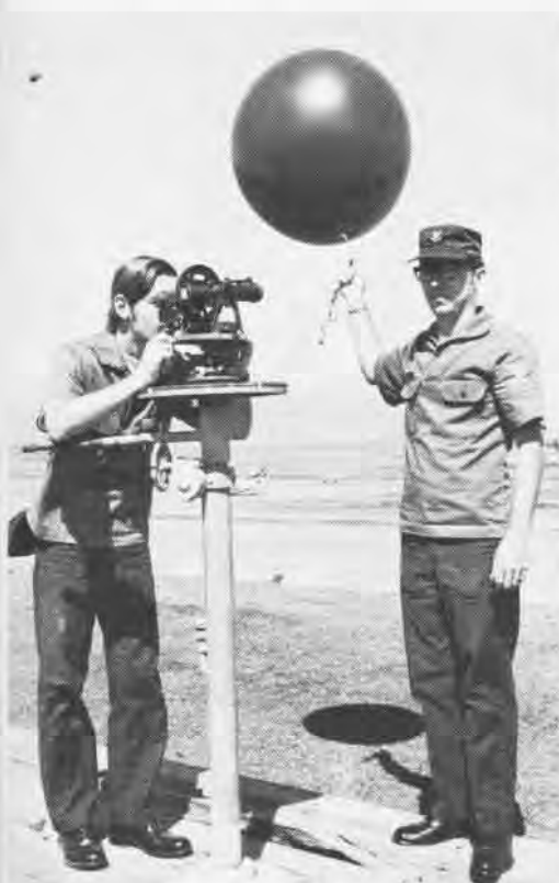
It's all in a day's work for Navy's weathermen. From left: doing administrative work; charting a storm's progress; running calibration tests on electronic equipment; checking alignment of theodolite before launching a balloon to gather data on wind speed and direction; checking wind speed and direction on automatic wind recording equipment; and briefing a Naval Aviator on weather conditions.
