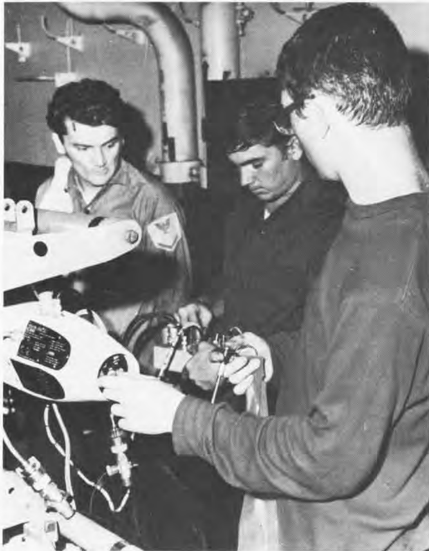
Prototype MER/TER tester is used during first fleet evaluation aboard Enterprise, above. Fins, electrical fusing, booster adapter and arming wires are installed during bomb assembly below decks, below. Enterprise AOs attach Mk 82 bombs to a MER, opposite top, and a flight deck bomb loader with his HLU-196 awaits delivery of a preconfigured load, right.
