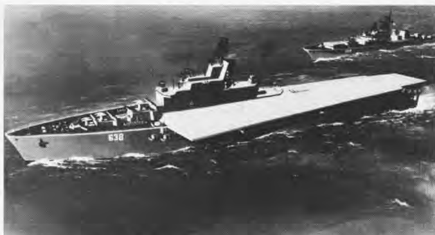
Above is artist's concept of the Soviet Union's first aircraft carrier. Under construction at the Nikolayev Nosenko shipyard on the Black Sea, the carrier is estimated to be 900 feet long, displacing approximately 46,000 tons. No catapults are in evidence, so it is presumed she will carry V/STOL aircraft. The new aircraft carrier is likely to be fully operational in a year. Two Soviet helicopter carriers, Maskva and Leningrad , are presently in commission.
