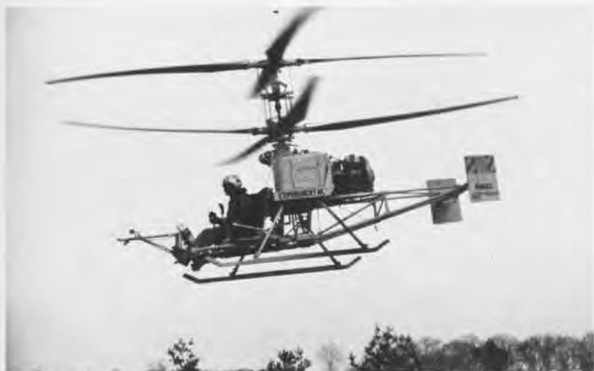
First flight of eight-blade coaxial rotor system on company-sponsored test bed aircraft was made by Gyrodyne recently using Navy-loaned components. Previous widely used Gyrodyne helos had four-blade coaxial rotor systems. Eight blades promise advanced helo concepts.
