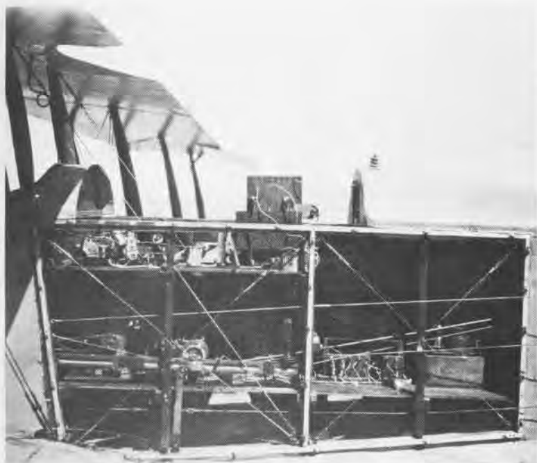
Inside view of automatic pilot and radio control equipment installed in N-9 seaplane at NAS Dahlgren, Va., November 1924. Below, with human pilot at controls, TDN assault drone is tested.
