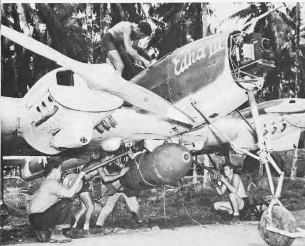
A TDR-1 is prepared for an attack somewhere in the Pacific. Note the television camera in the nose.
