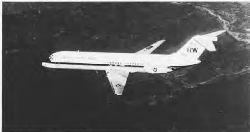
Navy took delivery of its first jet transport, the C-9B, on May 8. The Skytrain II is Navy's version of the DC-9 commercial jetliner. Its range, with a maximum payload of 32,444 pounds, is about 1,150 statute miles. Ferry range is about 3,400 miles and maximum gross takeoff weight is 110,000 pounds. The C-9B will accommodate a maximum of 107 five-abreast in its all-passenger arrangement or eight 88x108 standard pallets in an all-cargo configuration. In the combination cargo-passenger configuration there are seats for 45 passengers in the rear half. VR-30, NAS Alameda, Calif., and VR-1, NAS Norfolk, Va., will operate the transport.
