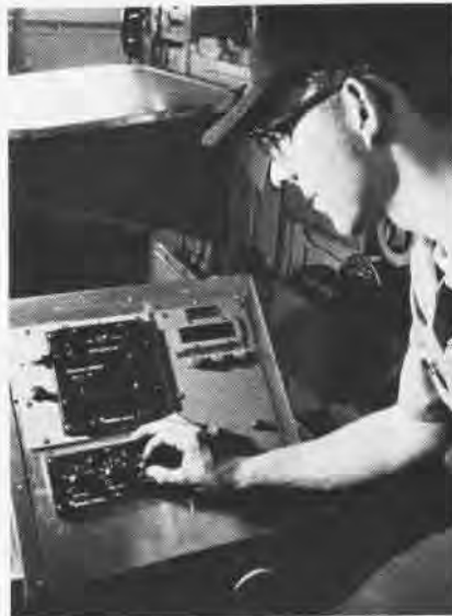
In Forrestal's new autopilot control area, QMSN Swatner sets the weather adjuster.
