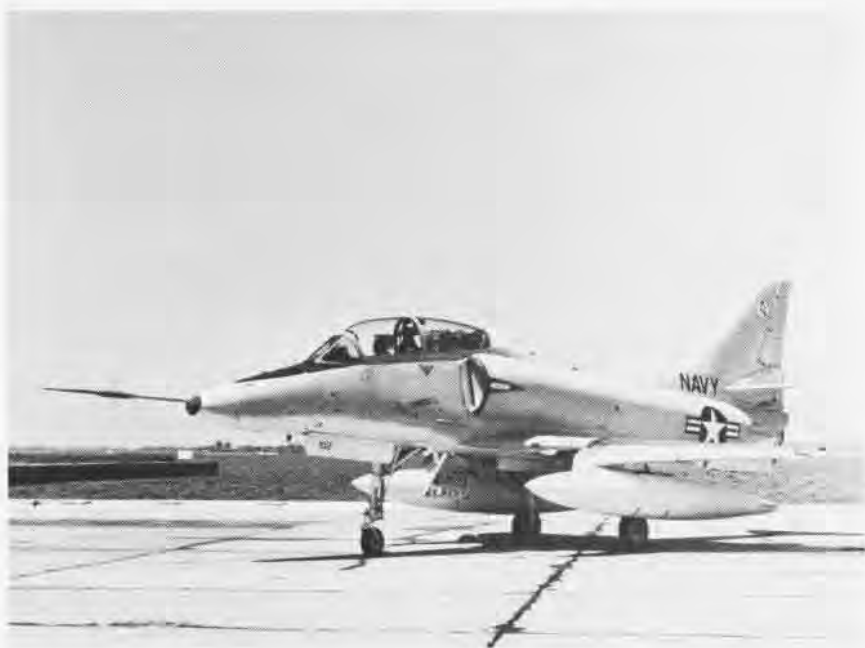
By using grid lines, the exact height of aircraft undergoing AIMS verification tests can be determined, left. Photo above is example of information which should be stenciled next to static pressure sources. At right is an instrumented A-4 with the special boom used for AIMS pacers at NATC.
