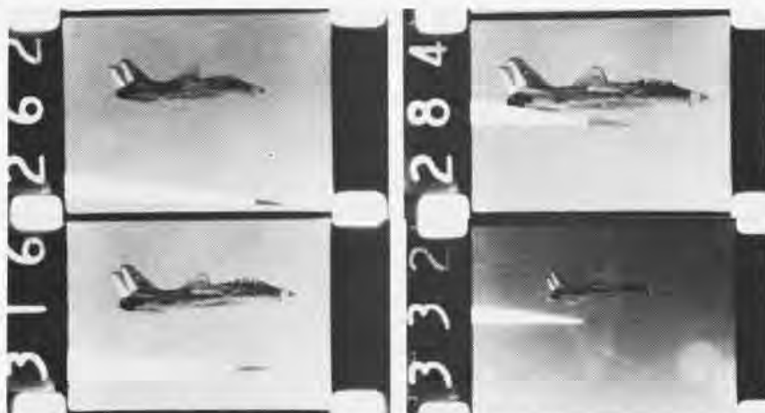
Four Phoenix missiles are launched within 44 seconds from an F-14 Tomcat during December 20, 1972, Navy test held at the Pacific Missile Range, Point Mugu, Calif. In the first four-missile firing ever attempted, the missiles scored four hits against four widely separated jet drone targets, each more than 30 miles away. Numbers indicate film footage, not elapsed time.
