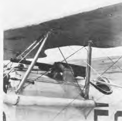
Browning .50 caliber machine gun, above, is mounted on a VE-7. The synchronizing mechanism leading from Hispano Suiza engine is visible below the barrel. A DH-4B, left, with its powerful 400-hp Liberty engine, was post-WW I workhorse.
