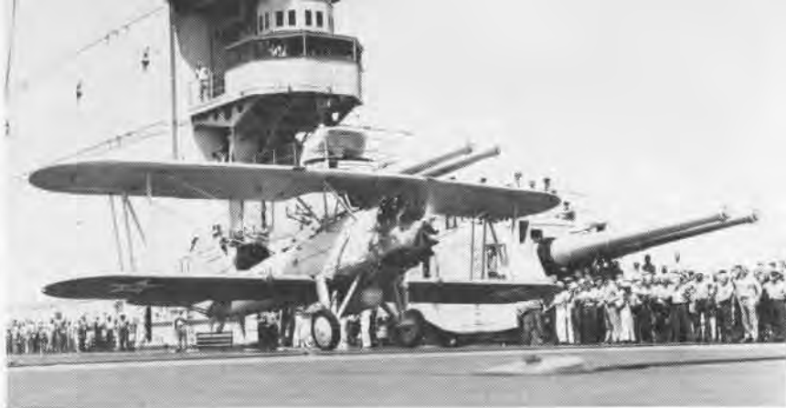
BM-1 draws a sizable audience as it takes off from stern of Lexington (CV-2) in 1934, right. Eight 8-inch guns supplemented Lex's aerial punch. Below, F6C-1 warms up on Langley's flight deck while the ship is in San Diego Bay. Hooks on axle engaged fore and aft cables on flight deck to aid in directional control.
