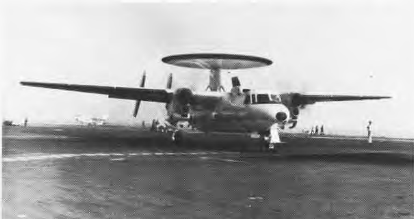
An advanced model of the Hawkeye makes its first carrier landing during recent carrier compatibility tests aboard USS America (CVA-66). The E-2C is expected to begin replacing the E-2B in a year. Main differences between the two models are more powerful engines, all new electronics equipment and an elongated nose which lengthens the aircraft by about two feet.
