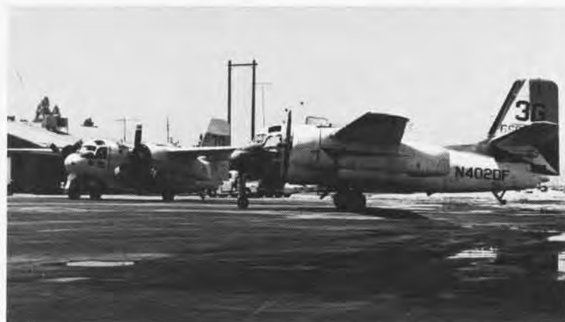
Opposite, Jeb Stuart disembarks from an Avenger following a fire-fighting mission. Above left, retardant is loaded into a PBY; leaks due to improper seal, above, were later repaired. Super Cats have 1,400-gallon capacity. Traker, left, has been converted to tanker at Ryan. Recently received S-2 on right awaits modification. Below, F7F-3 Tigercat takes off with bellyful of retardant.
