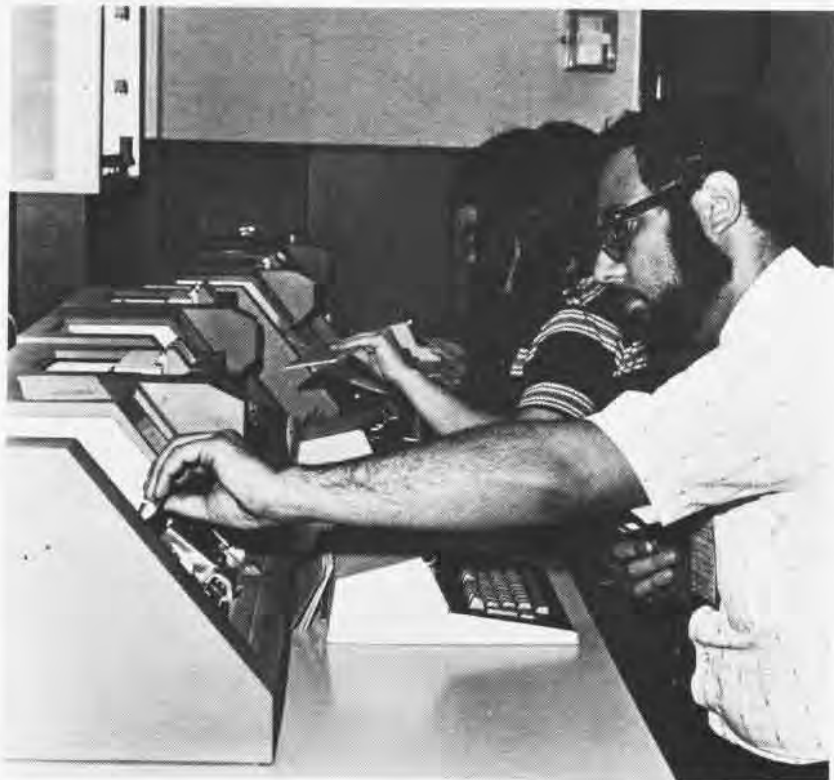
Ron Carriola, project engineer for the flightless bird explained the operation. "This is where the simulation process begins: with an engineer at the keyboard of a key punch, punching onto cards the equation/problem that he wishes simulated. The cards are then placed in the card reader which introduces the desired simulation to the computer."
