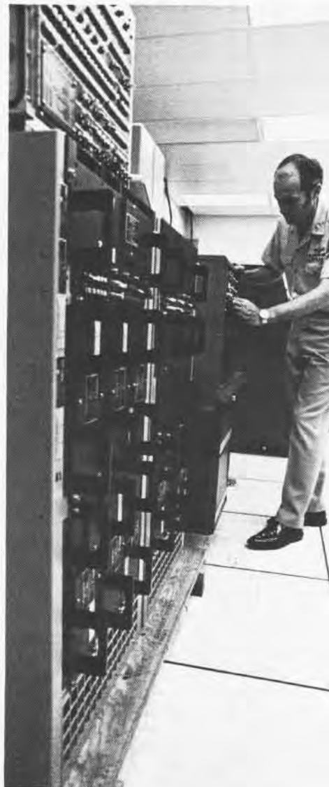
Future tactical support center watch officers will sit at main control consoles such as the one at center above. LCDr. Richard Fidler adjusts an AN/UYK-20 prototype mini-computer, above; in the foreground is the UYK-7 main TSC computer. Engineers work on a computer tape unit, far left. Equipment abounds in the TSC work area where technicians work with and check software programs, left.
