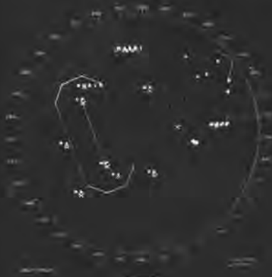
The radarscope is an essential part of the Navy Tactical Data System. The design on the left of the scope outlines a hazard area. Other symbols and numbers indicate the presence of aircraft or surface vessels.
