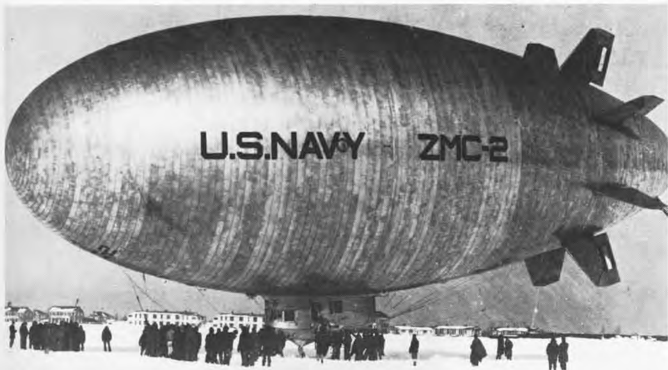
The Navy's ZMC-2, informally known as The Tin Bubble, was completed in 1929. Its unprecedented all-metal, 202,000-foot hide, executed in 0.0095-inch Alcad alloy, was of revolutionary design. Dismantled in 1941, the Bubble is being eyed as predecessor of airship design to come.
