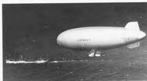
WW II K class saw extensive use in ASW ops; twin-engine, varied from 416 to 456,000 cu. ft.
