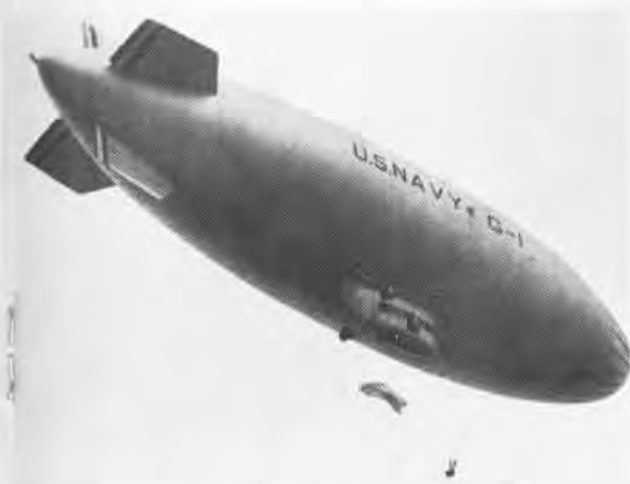
Twin-engine 178,000-cu.-ft. Goodyear G-1 was typical of between-wars non-rigids.
