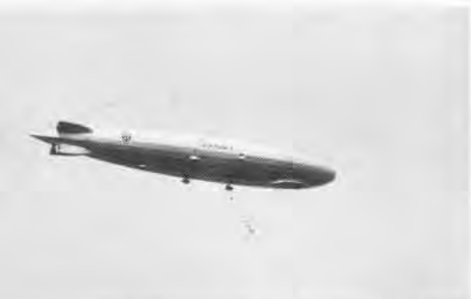
ZR-3, German-built Los Angeles, 1924, had five-engines, was 2,472,000-cu.-ft. dirigible.
