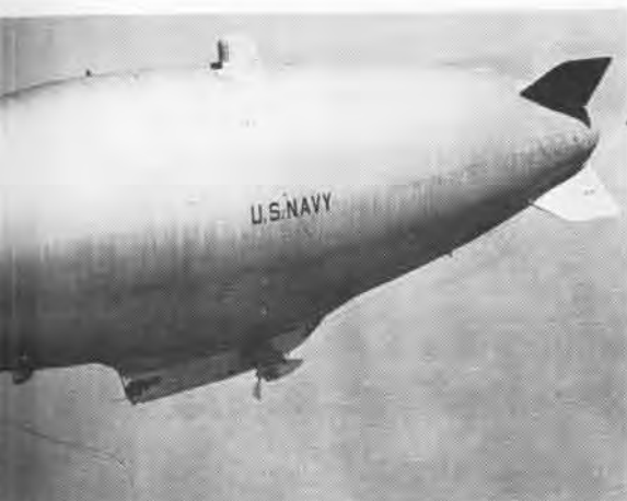
Postwar N class became widely used ZPGs; this is AEW ZPG-2W of over 1 million cu. ft.
