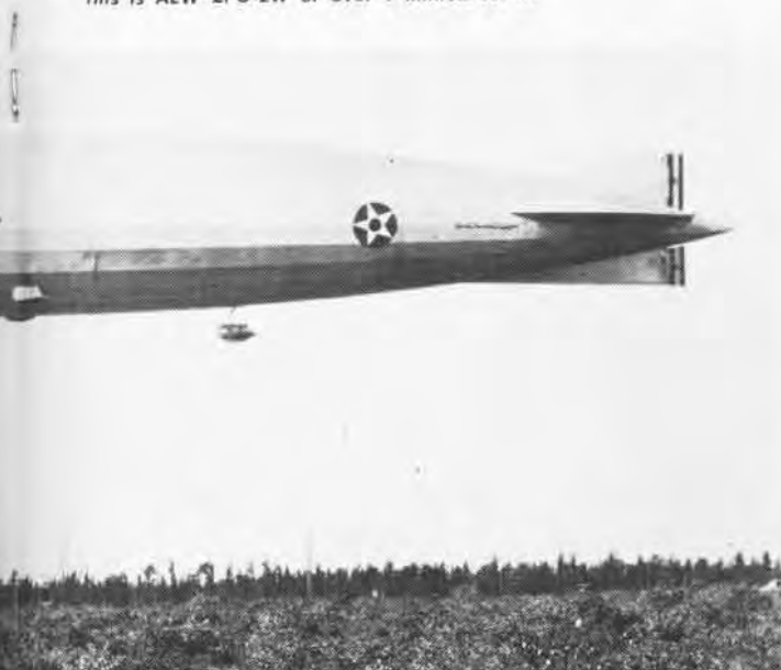
Postwar N class became widely used ZPGs; this is AEW ZPG-2W of over 1 million cu. ft.
