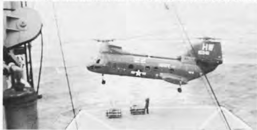
CH-46 Sea Knight conducts vertical replenishment for ship underway in Mediterranean Sea.
