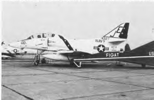
This fiberglass aerial target is towed for fleet gunnery exercises.
