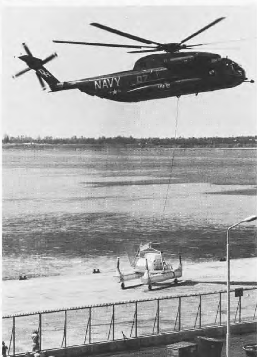
Mark 105, towed by helicopter, simulates the magnetic field of a ship by generating electricity which actuates the firing mechanism of magnetic mines.
