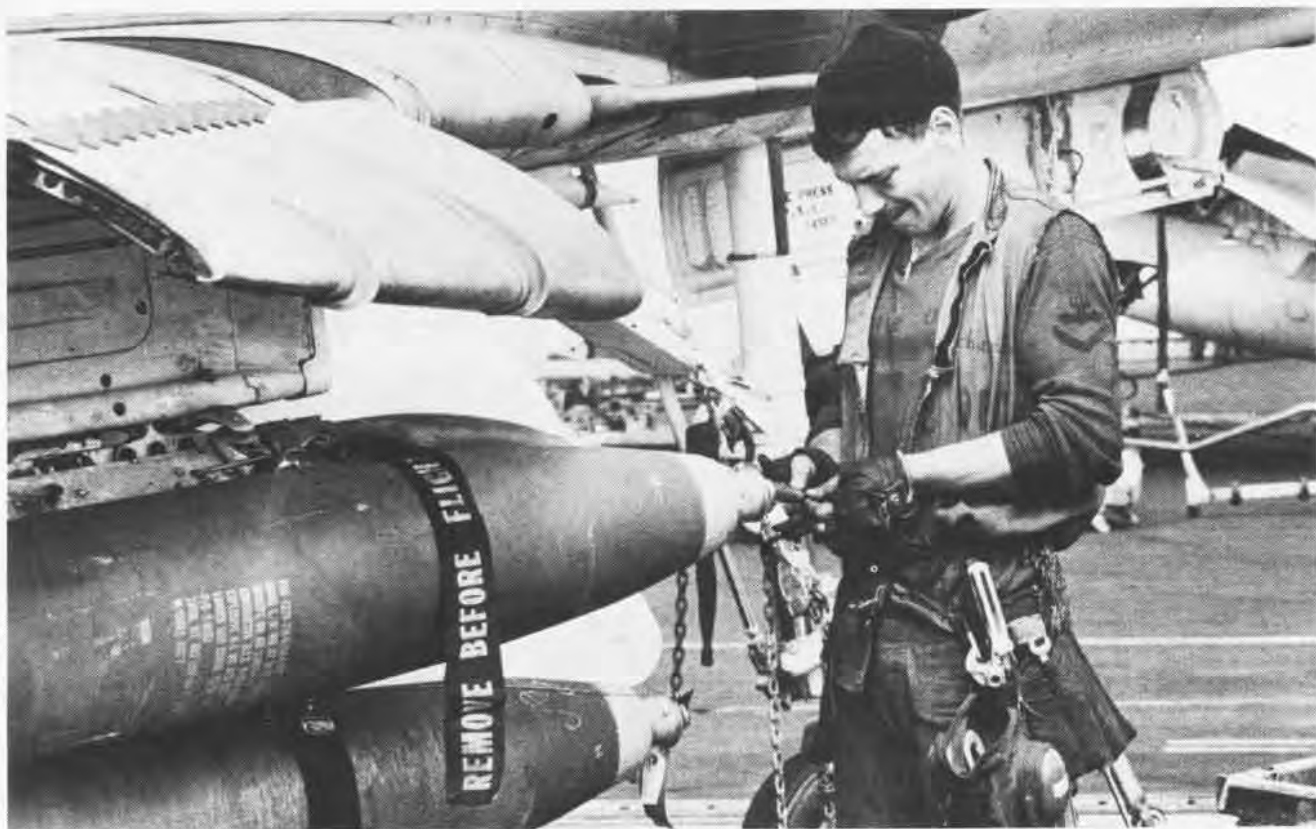
Ordnanceman pushes a skid of MK-81s during the rearming cycle, left. Fahnstock clips are installed on the arming wires during a load, above. Door gunner gives his M60 a final inspection prior to launch, right. The high-explosive, armor-piercing 20mm cartridges can be fired in 4.2 seconds when the three MK-4 gun pods are fired simultaneously, below.
