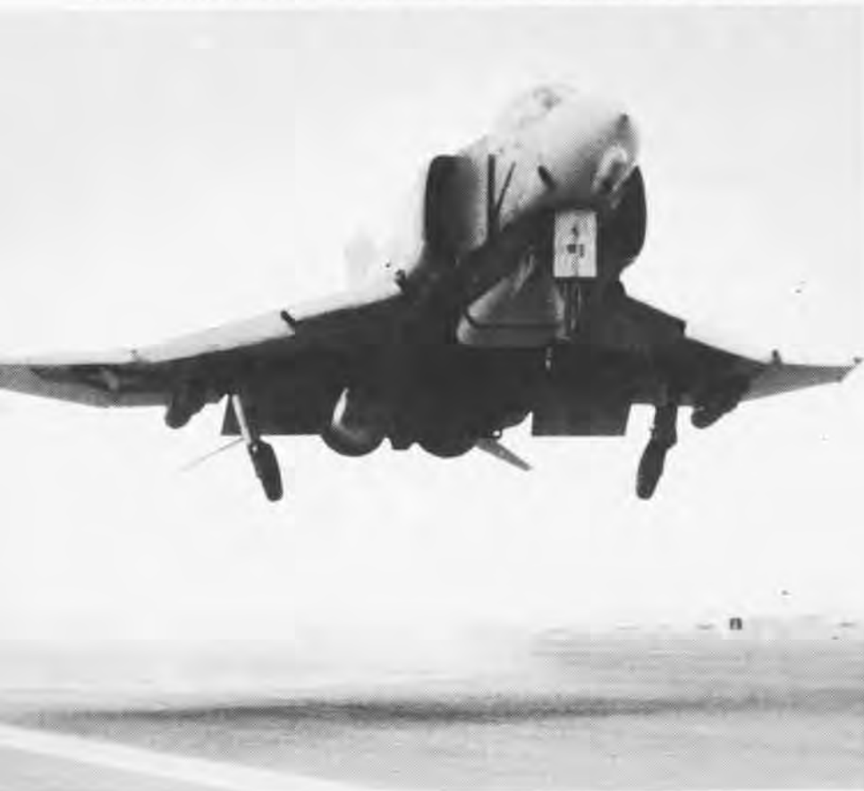
Phantom lifts off with simulated weapons load on conformal carriage flight test, below. Center, artist's concept of high-length-to-beam ratio surface effect ship of the future.
