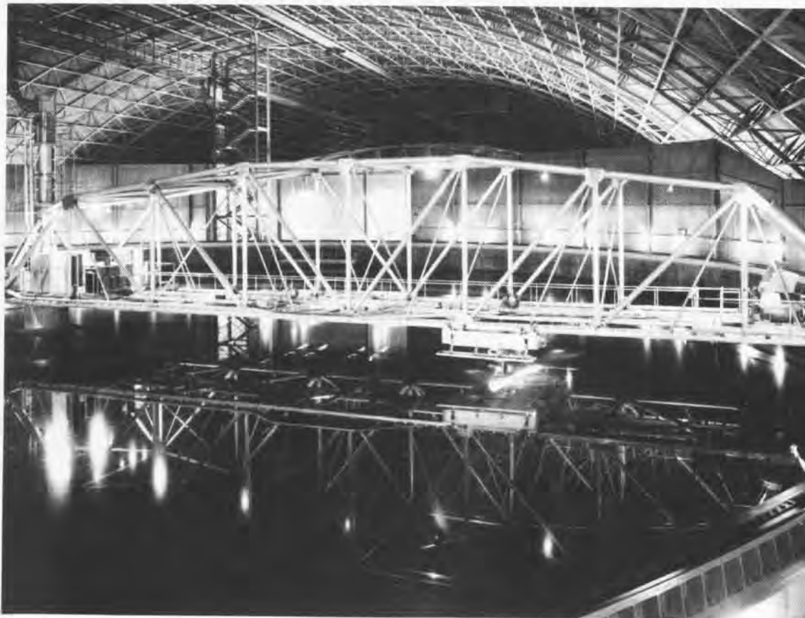
Rotating arm of the maneuvering and sea-keeping basin can move test models at comparatively high speeds. Simulated sea states are achieved by use of pneumatic wavemaker.
