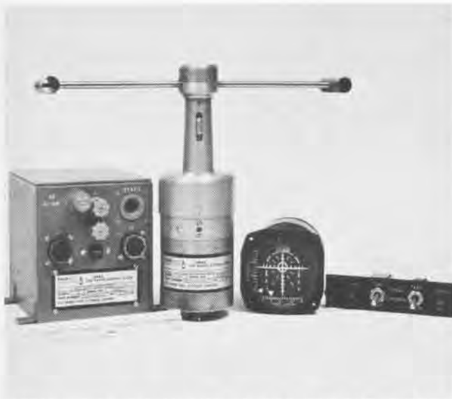
LORAS includes (left to right) air data computer, omnidirectional airspeed sensor, display unit and control panel.
