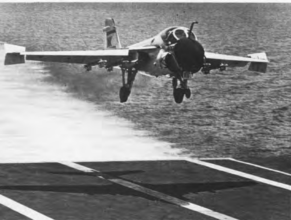
Top, during level run, bomb is released on practice target. Like "weird gaping mouths" the wing tip speed brakes help stabilize A-6 on approach to carrier deck, above. Opposite page, left, Intruder has compact but comfortable cockpit and provides good visibility. A-6s pass over cloud deck en route to USS Kennedy.
