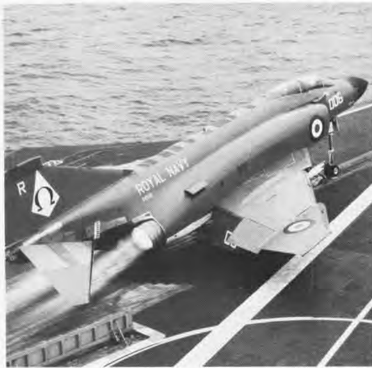
An F-4K in maximum reheat is about to be fired off Ark's bow cat.
