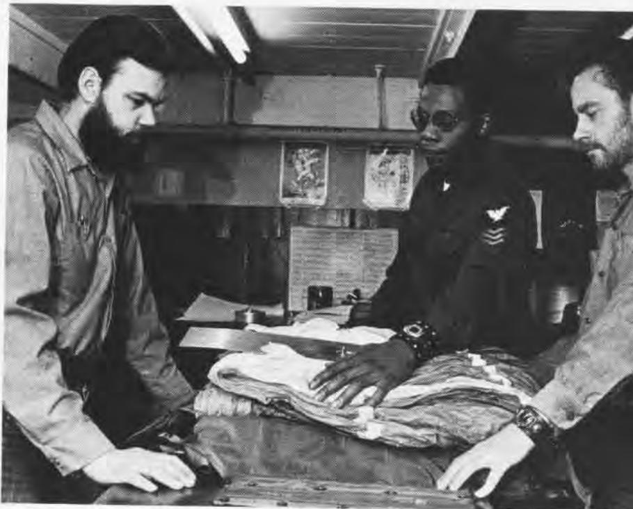
Parachutes packed by IMA personnel, top, will be delivered to the squadron paraflot to be stacked, checked, folded and repacked. After the whip and fold cycle, opposite, the quality assurance inspection, below, must be completed before the packers can continue placing the parachute panels and shroud lines in the backpack parachutes.
