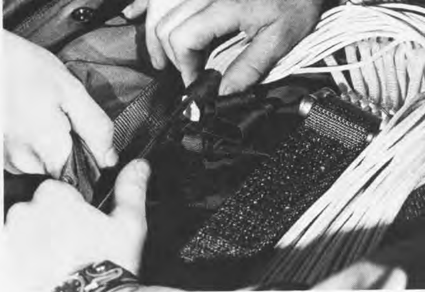
Lines are stowed in hesitator loops with a sewing hook, right. PR trainees at NAS Lakehurst line up for their first jump, below.
