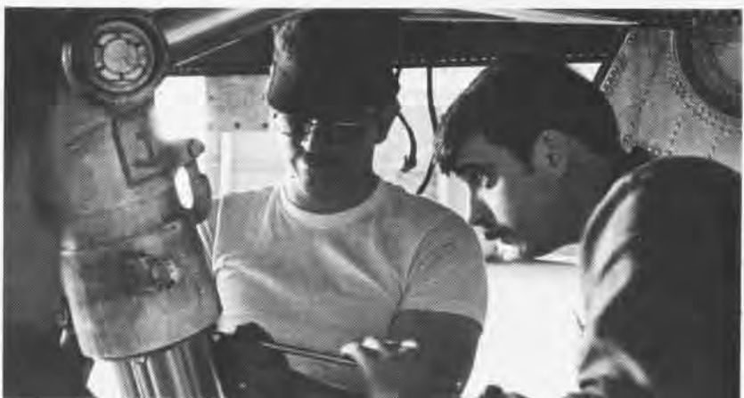
Phantom crew prepares to taxi out for weapons training flight, top. Middle, ground crew checks bomb rack prior to launch; rocket pods are positioned in foreground. Marines check landing wheel strut on squadron F-4, above.
