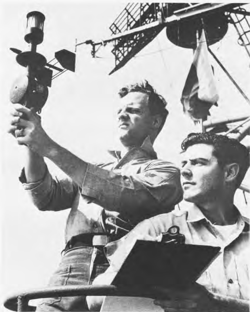
Aboard Hancock, AG3 Jim Sanders and AG3 Ken Blair read the winds with an anemometer, above. Another hand instrument indicates humidity and temperature.
