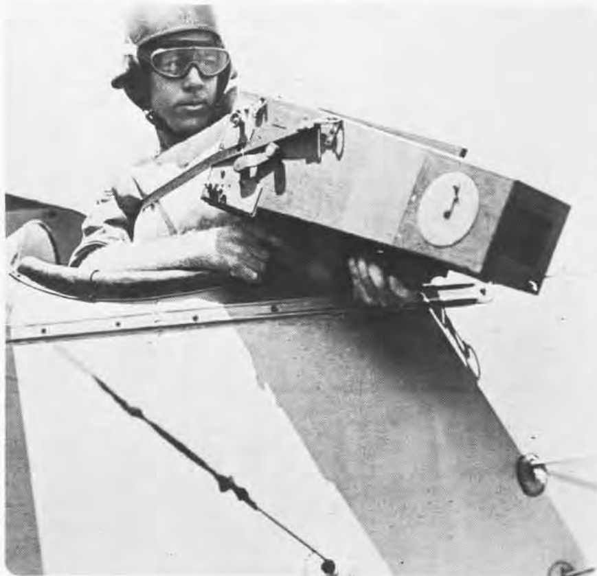
Ltjg. Richardson used this Eastman Kodak A-1 aerial camera aloft in 1919.
