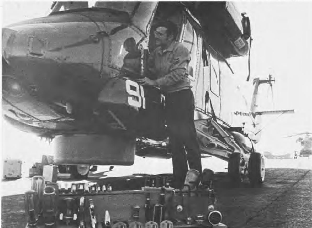
AM2 Matthew Greenlaw, HSL-30, adjusts SH-2F flight controls as AMH2 Gary Miller, VAQ-33, lubricates aircraft's components.
