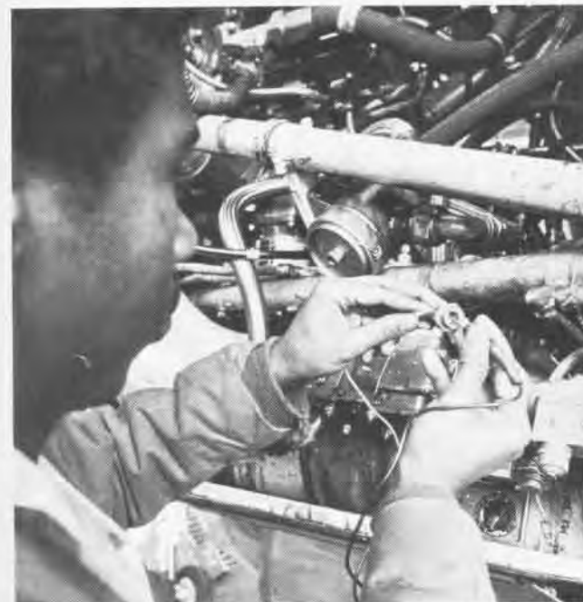
AE3 Robert Barrett inspects the fire protection wiring of a C-1A Trader. An AE must know the entire electrical system.
