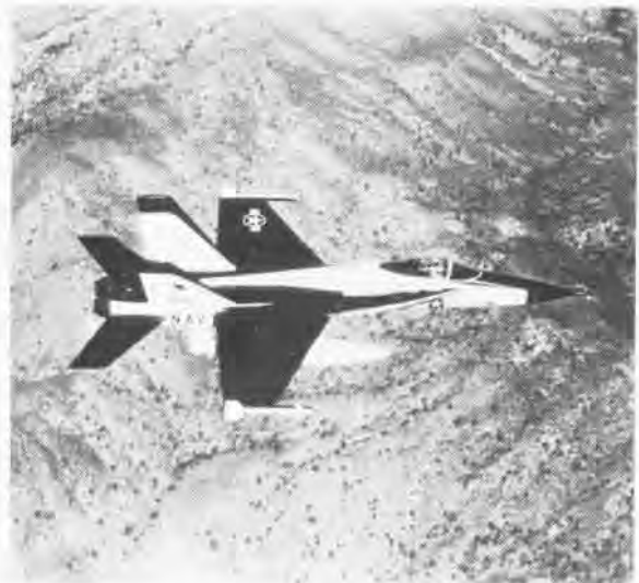
A-7 Corsair II, both of which it is designed to replace. The aircraft will carry Sidewinder and Sparrow missiles and an M61 20mm gun mounted in its nose.
