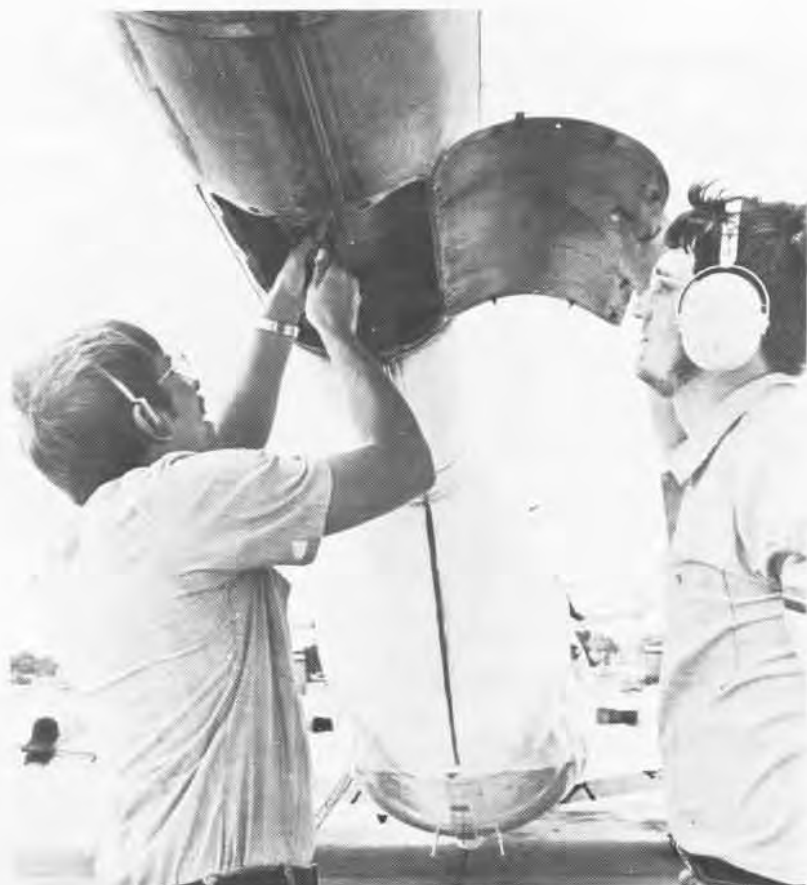
AX2 Robert Manning (left) inspects MAD gear in P-3C tail section as AX2 Randy Downs looks on. Below, A VS-22 Viking, MAD boom extended, keeps submarine under surveillance. Opposite page, close-up of AX trouble shooting cable contacts.
