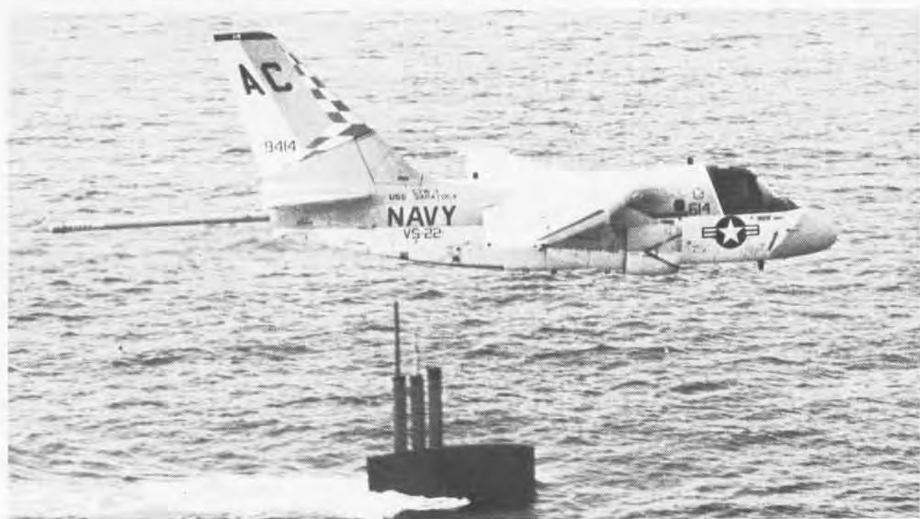
AX2 Robert Manning (left) inspects MAD gear in P-3C tail section as AX2 Randy Downs looks on. Below, A VS-22 Viking, MAD boom extended, keeps submarine under surveillance. Opposite page, close-up of AX trouble shooting cable contacts.
