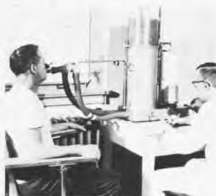
Depth perception was tested during the 1940 evaluations by using frontal plane apparatus consisting of a hinged board which the subject manipulated with pulleys to line up the images. Aspiratory air flow was measured for the first time in the 1963 lung function test.
