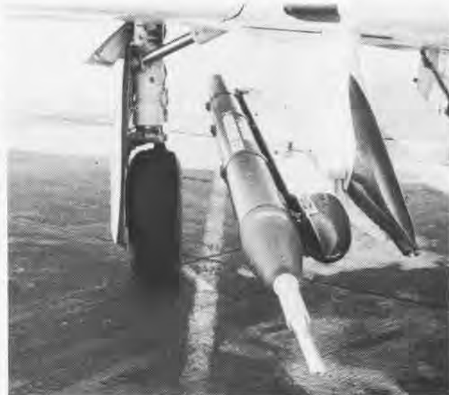
AIS pod mounted on LAU-7 launch rail, above. Opposite center, aerial view of an F-5 being tracked by an F-14. Photo courtesy of Grumman Aerospace. Small photos are of range mission data which is at the finger tips of the instructor at the DDS control console.
