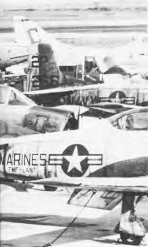
Preservatives make these birds look worse than they really are as they wait at Chevalier Field for their turn in the rework cycle. To the left, but not shown, are NARF's newest additions — a $5 million assembly building and an $8 million cleaning and disassembly facility.
