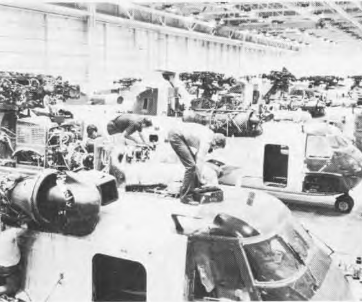
Workers reassemble H-53 and T-39 in Rework Two as sheet metal mechanic repairs inside of A-4 tail section. T-39 skeleton, set in a jig to prevent frame warping, shows rework required due to excessive corrosion.
