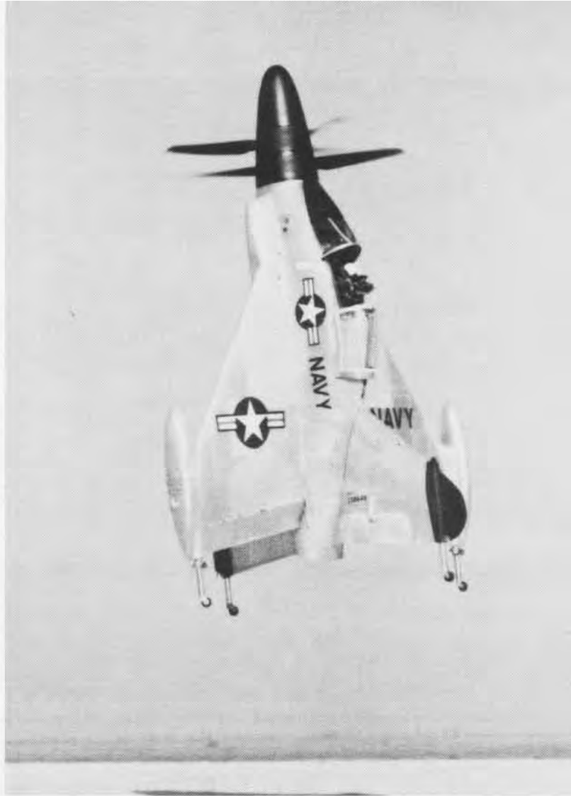
Marine AV-8A is U.S.'s first operational V/STOL plane, above. Convair's XFY-1, from another generation, was a tail-sitter type, right. Below, in the Ames Research Center wind tunnel is Navy/NASA lift/cruise fan research model.
