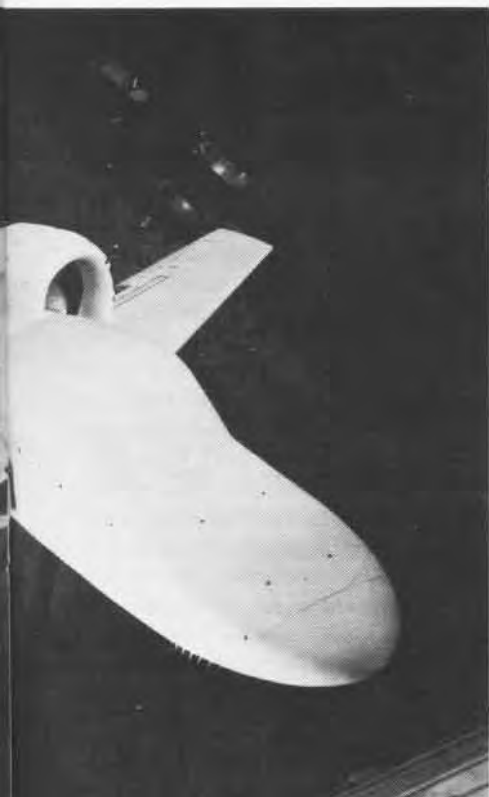
Top view shows Boeing V/STOL A concept with lift/cruise fans. Above is Rockwell XFV-12A, real-life version of which is being tested.
