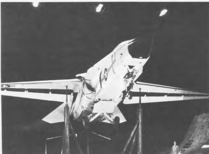
Some aircraft which have spent time in the Forty-by-Eighty's test section are the F-111, undergoing tests, gear-down, below; the YOY-10 STOL research aircraft, right; and, above, a remotely piloted research aircraft with a swivel wing. Aircraft are prepped on the test chamber floor, then raised and positioned on the variable-height support struts. The tunnel's test section is 80 feet long, 40 high and 80 wide. Scales can measure 90,000 pounds of lift and 16,000 pounds of thrust or drag. Engines, prop or jet, can be running during the tests, as with the OV-10A, right.
