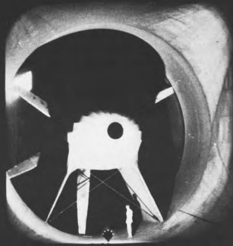
Each of the tunnel's electrically-driven motors has 40-foot-in-diameter, six-bladed fans and generates 6,000 horsepower. Combined, they produce an airflow which reaches a peak velocity of 250 miles per hour through the test section.
