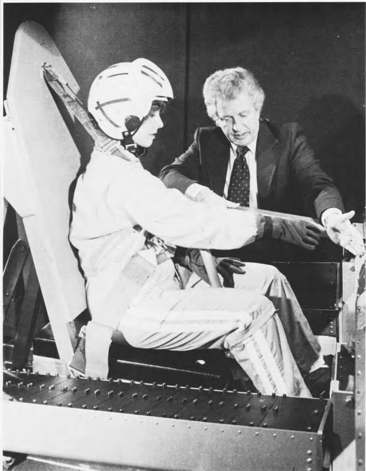
Dr. Robert Delvecchio checks arm reach of Stephanie Meyer in the reconfigurable crew station evaluator.
