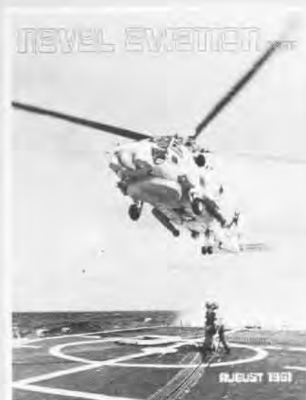
COVERS — Front, SH-60B prepares for hookup to the RAST system aboard USS McIntnerney. Back, final landing phase as viewed from McIntnerney's helicopter control tower.
