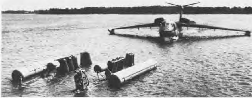
Beaching cradle could be engaged or disengaged without assistance from beaching crew. The P6M could taxi into or out of water when locked in cradle.
