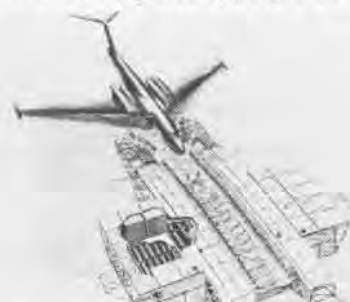
Drawing shows one means by which P6M aircraft could be dispersed to operate from remote locations. This support platform idea envisioned a relatively inexpensive floating base which could be towed from one location to another.
