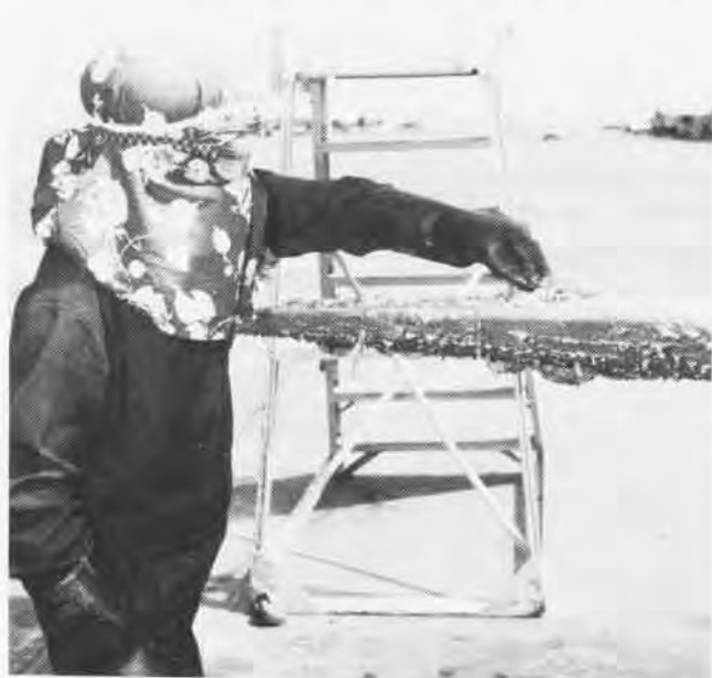
Top left, aerial view of Naval Air Station, Cubi Point. Top right and above, stripping paint from an RF-8G.
