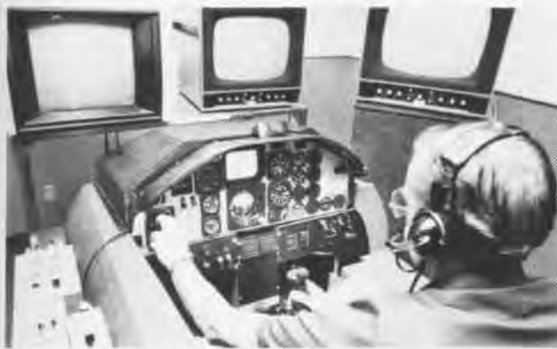
Far left, BQM-34A Firebee drone used to tow targets for gunnery exercises. Left, drones will be controlled eventually from a cockpit simulator using nose camera video information. Below, Sam Doran keys a left rudder signal on his remote control console to correct takeoff roll of QF-9 target drone at NAS Point Mugu.
