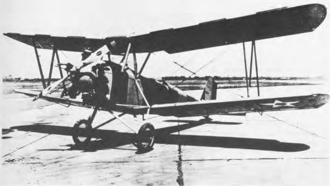
Left, the TDN was the first aircraft built specifically as a drone aircraft by the Naval Aircraft Factory, Philadelphia. Above, a 1930 New Standard NT-1 trainer converted to a drone by the Naval Aircraft Factory in 1937. Below, a 1938/9 drone converted from a Curtiss N2C-2 trainer. Originally a tail dragger, a nose wheel was installed on this aircraft for easier handling by the remote control operator.
