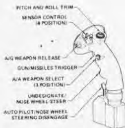
Above, cutaway view of the weapons tactics trainer. Left, schematic views of stick and throttle showing HOTAS functions incorporated into the part task trainer. Below, F/A-18 cockpit showing cathode ray tubes with alphanumeric displays.
