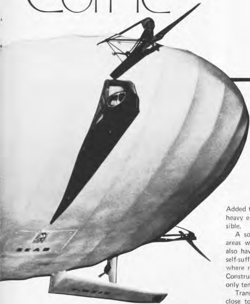
French-built, lenticular-shaped hybrid vehicle for heavy lift and general utility.
