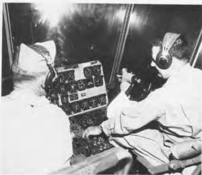
Cockpit view of a ZPG-3W. The N-series blimps were the first nonrigid airships to have controls similar to those of an airplane.
