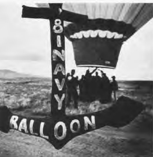
On the Navy balloon, an anchor holds down the line used to stretch out the craft during the deflation process.
