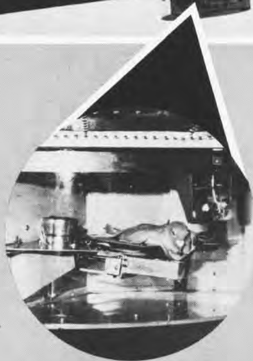
Coast Guard helo with pigeon observation chamber underneath. Pigeon is resting on special couch in compartment.
