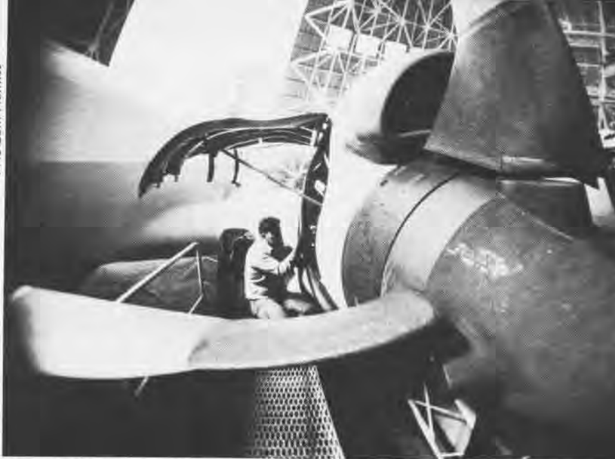
Exaggerated by the superwide angle camera lens, a VP-31 mechanic checks a turboprop engine on one of the squadron's P-3 Orions.
