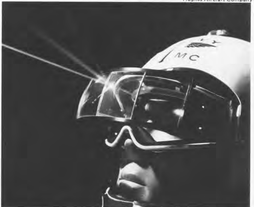
The experimental visor, shown here on a mannequin, is produced in separate segments. Production units would be constructed in one piece for mounting on an aircrewman's helmet. The visor could also be produced as eye protection goggles for ground personnel.
