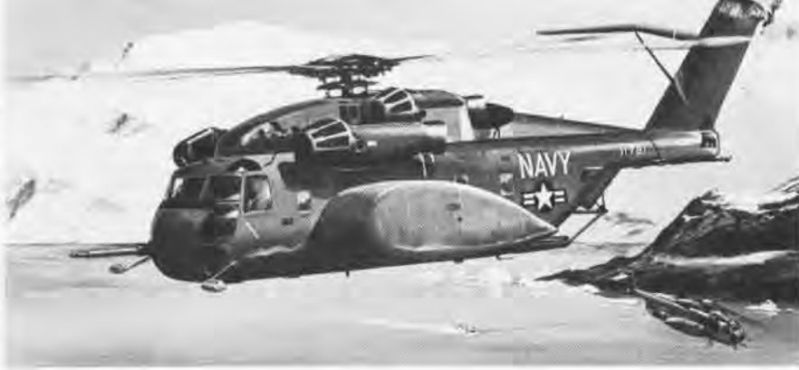
In an artist's concept, the MH-53E Super Stallion is seen in flight during minesweeping operations. Note enlarged fuel sponsons adding to on-station time.
