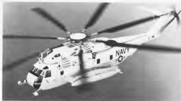
The CH-53E prototype of the mine countermeasures version flies during testing by Sikorsky.
