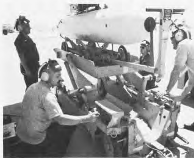
Loading an ALE-41 chaff pod takes a lot of coordination and mechanical muscle.
