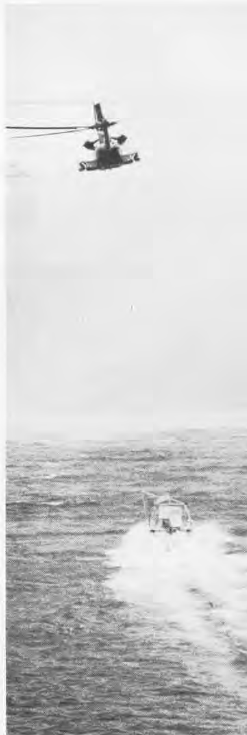
With the sled up on the foils, an HM-16 Super Stallion prepares to sweep the harbor entrance to Halifax, Nova Scotia, for mines during a joint Canadian-U.S. exercise.
