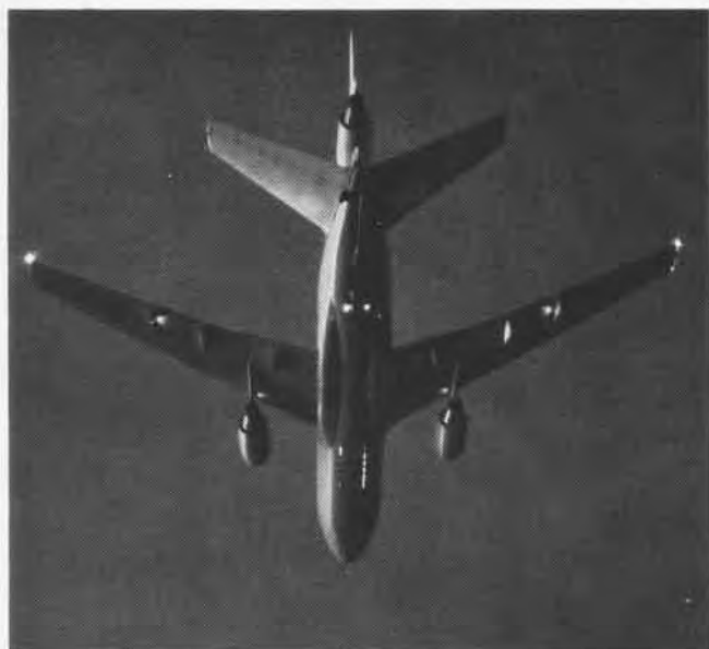
The underside lighting array of the KC-10 provides an excellent visual reference during approach under low visibility conditions.
