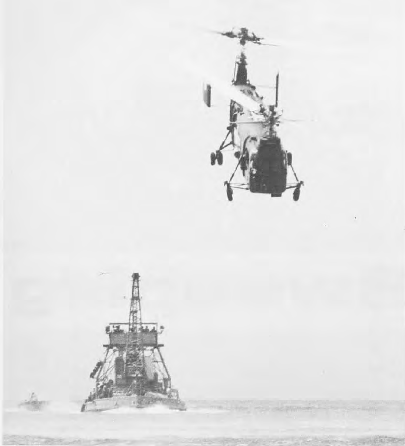
An HSL-1 tows a heavy load during the 1956 evaluation of towing characteristics. Note the extreme nose-down attitude of the helicopter.
