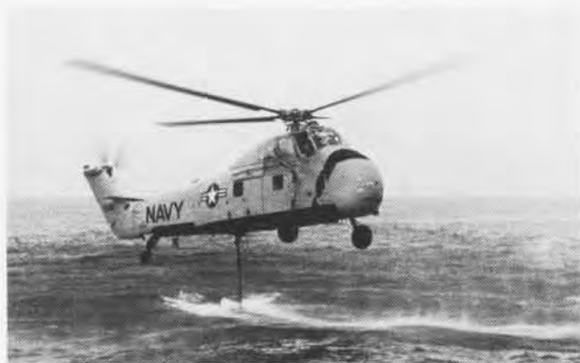
The HSS-1 Seabat, in 1958, was the first single-rotor helicopter tested as a mine countermeasures vehicle.
