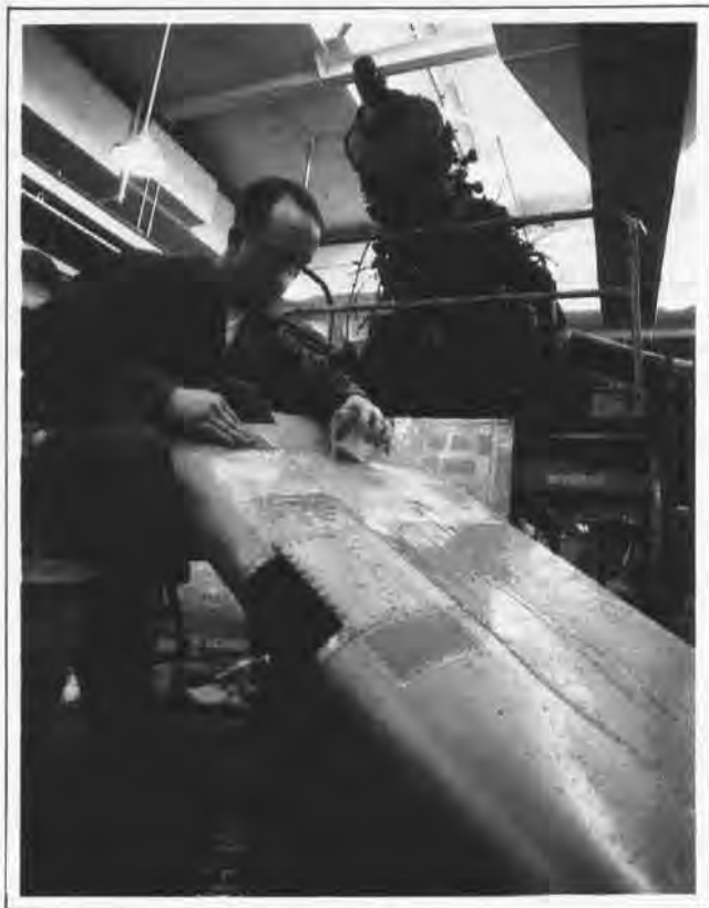
Attention to detail is a cornerstone of the aircraft restoration program. Here, LCpl. Stan Pate applies muscle and tender loving care to remove corrosion from an F4U wing control surface. Below left, a collection of antique, wooden aircraft props glow under the museum lighting.
