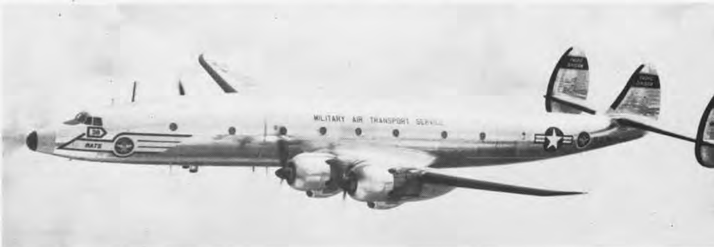
Above, an R7V-1 Constellation bears the markings of the old Military Air Transport Service. Left, a WV-2 airborne early warning version of the Super Constellation sports the "flying saucer" radome in 1956.
