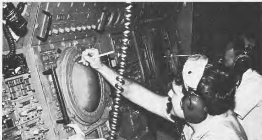
An RVAW-120 Naval Flight Officer (NFO) student learns to use the Light Pen Hooking Marker (LPHM) in the 15F8 Tactics Trainer.
