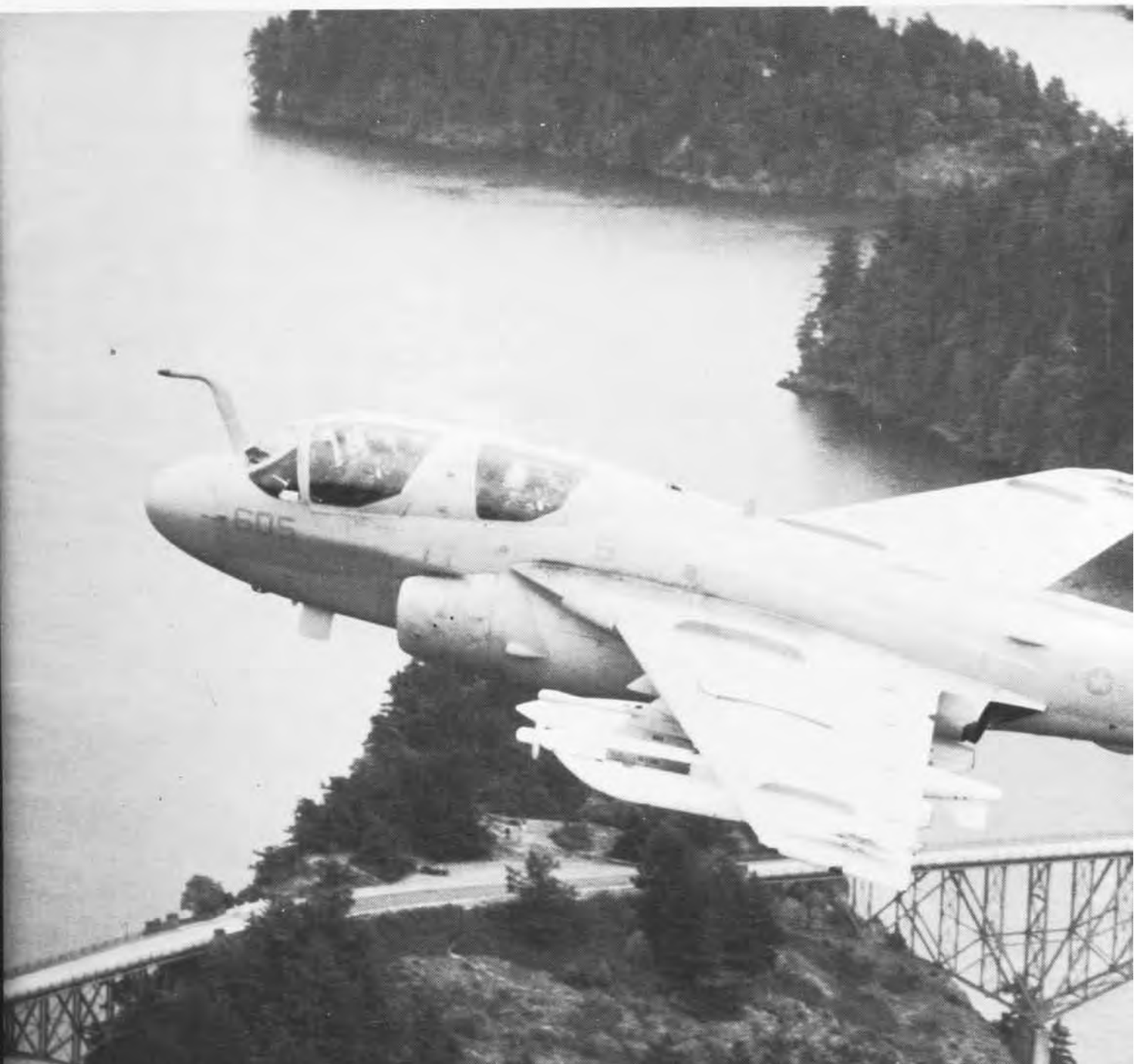
Grumman's prototype of the Navy's Increased Capability II (ICAP-2) version of the EA-6B Prowler flies over Deception Pass near NAS Whidbey Island during aircraft trials in early 1982. With several sophisticated interfaced computers, the ICAP-2 Prowler will offer an increase in high-speed information processing to respond to a detected environment. The new equipment includes the Navy's new standard AYK-14 computer. The aircraft is expected to become operational in 1984.
