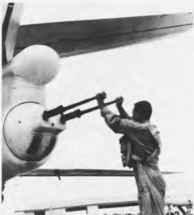
The 20mm radar-guided cannon in an A-3 tail are checked prior to flight. Heinemann considered it excess weight, but the Navy insisted on the weapon for tail defense. The cannon was eventually removed by the early 1960s.
