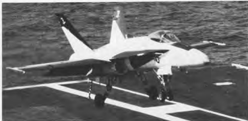
An F/A-18 takes the wire for an arrested landing aboard the Navy's newest nuclear-powered aircraft carrier, Carl Vinson. McDonnell Douglas Corporation
