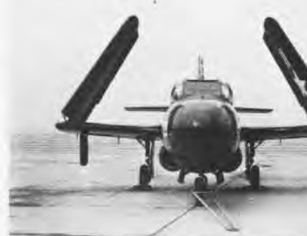
This front view of the XF3D shows the extra wide cockpit in which the pilot and enlisted systems operator sit side by side.
