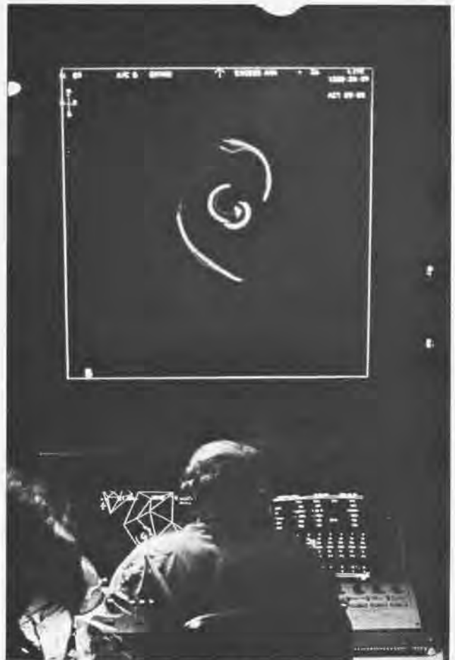
Inside the Tactical Aircrew Combat Training System (TACTS) van at MCAS Yuma, an air-to-air dogfight is depicted on the monitor screen. The display is created from signals transmitted from electronic pods attached to the fighters, and recorded for replay later.
