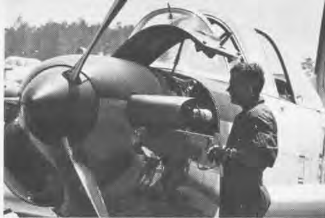
Ensign Mike Reiter preflights a T-34C at NAS Whiting Field, learning more than 80 specific checkpoints, to his instructor's satisfaction.
