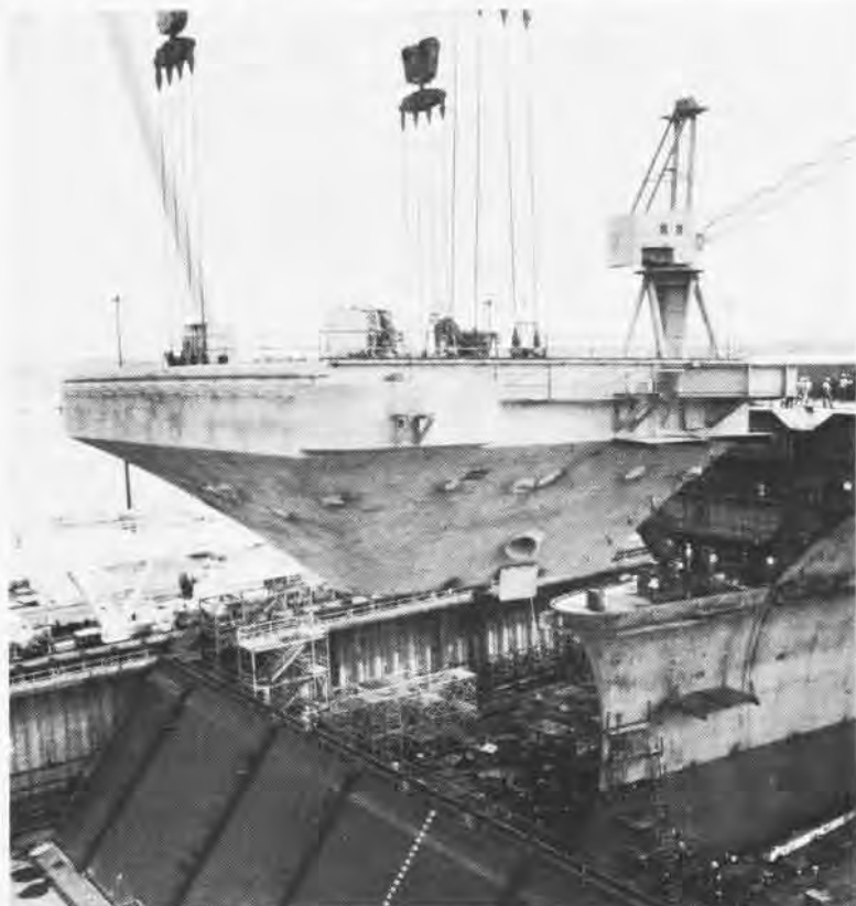
Above, Roosevelt attains her full length as new superlift crane lowers 700-ton bow section into place.
