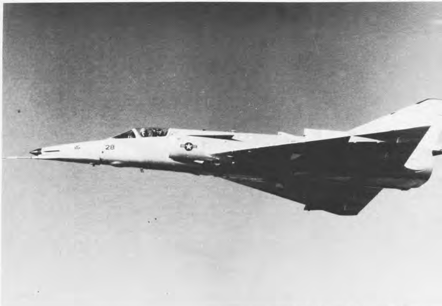
The Israeli-built Kfir, designated F-21A by DOD, is a Mach 2-plus, single-seat tactical fighter powered by a single GE J79 engine.
