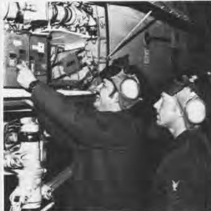
AQ1 David W. Wear, USNR-R(TAR), left, and AT2 William L. Forstner, USN, work side by side removing one of the AWG-9 weapons systems computers.
