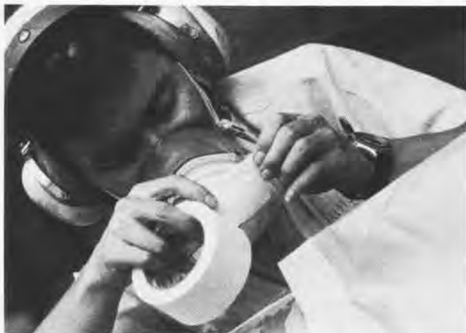
Top left, AMS3 Russell Rulona tapes a border around a portion of an S-3A's wing before spraying it with paint. Top right, AD3 Eddy Formera, left, and ADAN Dominick Bulone, right, prepare to install a new S-3 engine into one of VS-41's aircraft. Bottom, a squadron plane captain prepares to taxi out an S-3.
